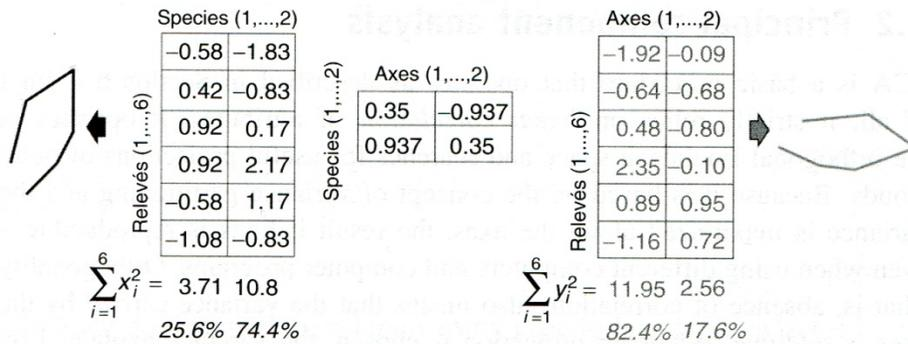
**Figure 6.4** Numerical example of PCA. The centred data matrix (left) is multiplied by the matrix of eigenvectors (centre) to yield the ordination coordinates (right). The variances of the ordination axes are the corresponding eigenvalues.
